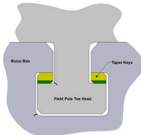
**Figure 2 above shows a Tee head attachment of the rotor pole to the rotor rim.**
