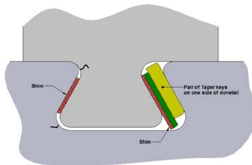
**Figure 1 above showing dovetail attachment to the rotor rim.**
