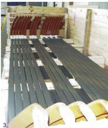
(1) Tooling for coil shaping and curing is developed from the engineering design using 3-D modeling. (2) Prototype coils undergo tests at various stages of manufacture. (3) Coils are transported to site for storage in specially built crates.
