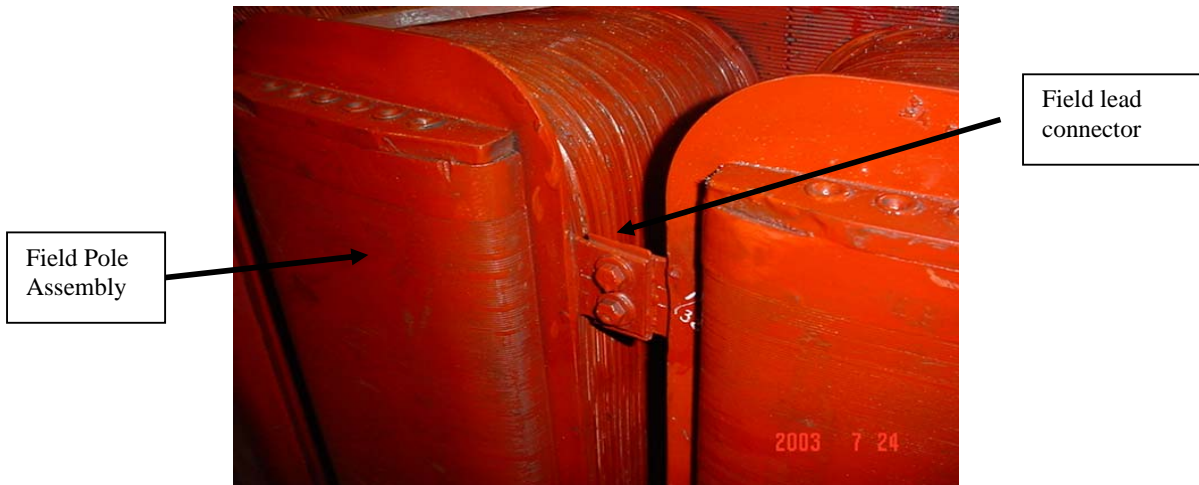
Fig. 1. Configuration of Field Winding Lead Connector
